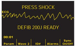
A continuous tone will sound for 50 seconds, followed by an intermittent beeping for 10 seconds. The shock must be delivered within this 60 second interval or the defibrillator will disarm itself.
