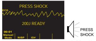
A continuous tone will sound for 10 seconds, followed by an intermittent beeping for 5 seconds. The shock must be delivered within this 15 second interval or the defibrillator will disarm itself. Press and hold the illuminated **SHOCK** button on the front panel until energy is delivered to the patient.
