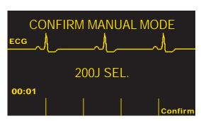
If the access code is not configured, the message "Confirm Manual Mode" and Confirm softkey will be displayed. Press the Confirm softkey to enter the manual mode of operation. If the Confirm softkey is not pressed within 5 seconds the unit will revert back to semiautomatic operation.
