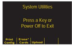
Note: Softkeys and messages denoted with an asterisk (\*) are displayed only if unit is configured to allow card erase.
